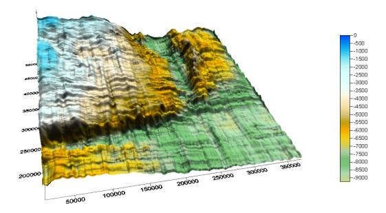
Figure 3. Basement of the Bishop model interpreted on every 10<sup>th</sup> row and column, using Enhanced 3D inversion. Rows and columns are spaced at 200 m, and a 6000 x 6000 m smoothing filter was applied to the final result.
