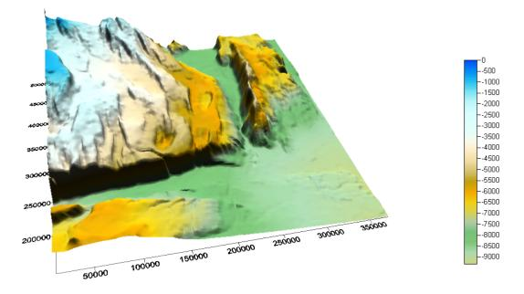
Figure 2. Smoothed Basement of the Bishop model. The model is based on real topography of an area in California, with susceptibilities assigned according to a simple model. The topography has then been transcribed downward to the depths (in m) indicated by the colour bar beneath non-magnetic sediments. There are no basement faults in the model. This image has been smoothed with a 6000 x 6000 m smoothing filter.
